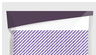
Diagonal sealing (seal width defect)
